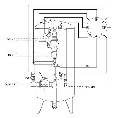
**Note:** When high iron content or turbid waters are encountered, put a small cartridge filter ahead of the stager inlet port.
